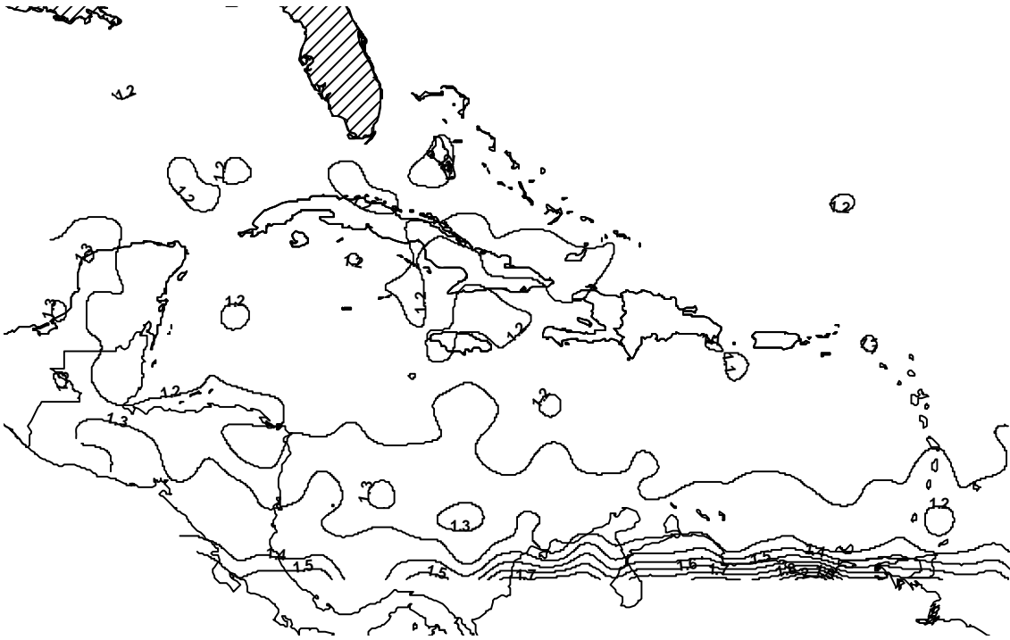
Figure B-3 Contour plots of importance factor for ASCE category III and IV structures defined by I=(V_{1700}/V_{700})^2
